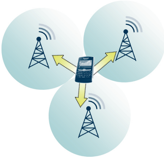
Fig. 5.11. Time Difference of Arrival (TDOA) positioning (GIS Development, 2006)
