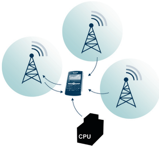
Fig. 5.12. Enhanced Observed Time Difference (E-OTD) positioning (GIS Development, 2006)
