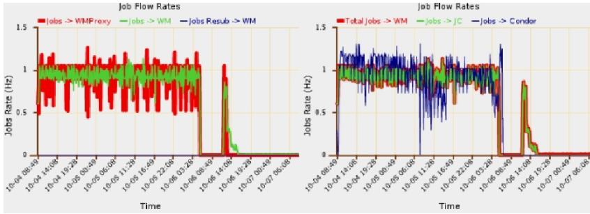
Fig. 2. Throughput of about 90.000 jobs/day (>1 Hertz rate as shown by the plot) over a period of more than two days on a stress test by CMS
