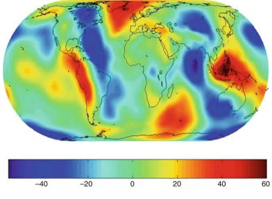
$\hfill Fig. 7$  The disturbance potential from EGM96 at height 250 km in  $m^2/s^2$
