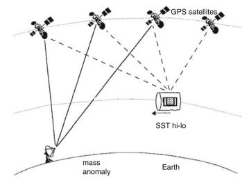
The principle of satellite-to satellite tracking (from ESA (1999))
