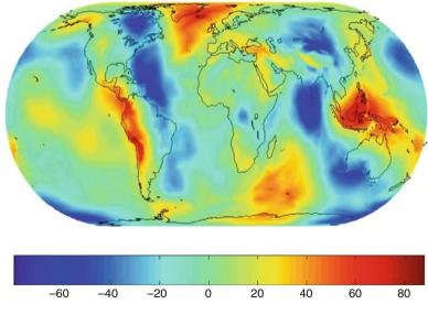
■ Fig. 6 The disturbance potential from EGM96 at the Earth's surface, at height 250 km, in m<sup>2</sup>/s<sup>2</sup>
