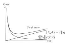
Fig. 9 Typical behavior of the total error in a regularization process
