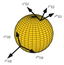
**G** Fig. 4 Local triads  $\varepsilon^r$ ,  $\varepsilon^{\varphi}$ ,  $\varepsilon^t$  with respect to two different points  $\xi$  and  $\eta$  on the unit sphere
