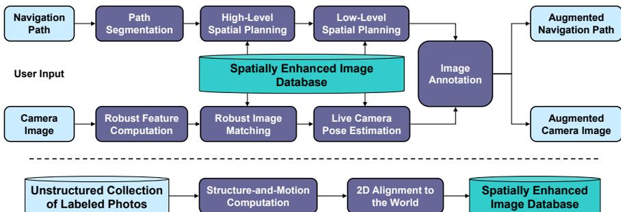
**Fig. 3.** Block diagram for landmark-based navigation supporting two modes: one that produces a set of augmented images for a user-supplied navigation path and one that augments a user-supplied image. Below the dotted line we show construction of the spatially enhanced image database from an unstructured collection of labeled photos.
