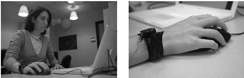
Fig. 1. Vibratory motor integrated into a bracelet to serve as a haptic feedback device
