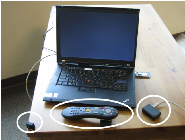
Fig. 2. Data Collection Components: top, a logging laptop; bottom from left to right, a video camera pointed at the room to gather ground truth about who was watching TV, a remote control with our accelerometer module attached, a universal infrared code receiver
