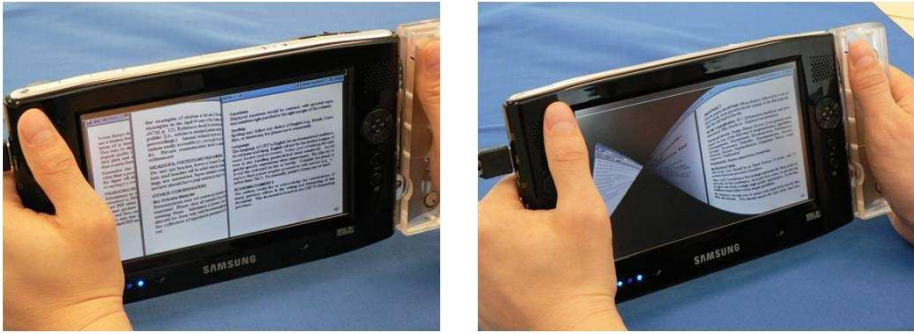
Fig. 3. Two examples of force-based interactions: (left) bending for page turning and (right) twisting for application-switching, with visual feedback
