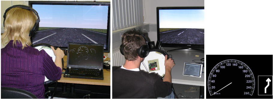
Fig. 2. Setup in the first study with the control panel on a laptop (left), setup in the second study with control panel on a 8'' display (middle) and a close-up of the control panel with an direction arrow used in the second study (right)
