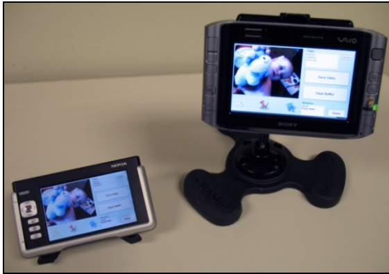
Fig. 4. KidCam's interface can be remotely viewed and controlled via another device ( i.e. , a Nokia Internet Tablet) that can replicate its screen and audio
