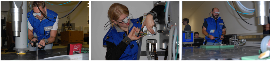
Fig. 6. Maintenance pictures from the experimental sessions. From left to right: Checking bearing pressure, installing the x-motor and y-gears.
