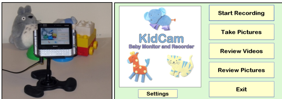
Fig. 2. View of KidCam prototype on a Sony VAIO (left) and a screen shot showing the main menu of KidCam's interface (right)
