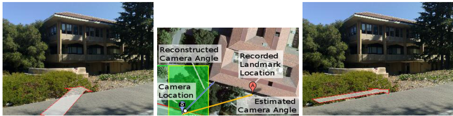
Fig. 5. An example of correcting image augmentation using reconstruction data. The goal is to specify a path which passes alongside the building. Compare the uncorrected case (left), which relies on GPS location of the camera and the landmark, to the case which uses the automatically computed camera pose (right). The center map shows the difference in camera angle between the two techniques.
