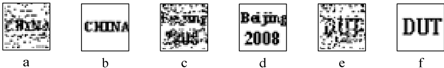
Fig. 3. Extracted blurred images and restored images. a. blurred watermark image 1, NHD is 0.1621. b. restored watermark image 1, NHD is 0. c. blurred watermark image 2, NHD is 0.1738. d. restored watermark image 2, NHD is 0. e. blurred watermark image 3, NHD is 0.1963. f. restored watermark image 3, NHD is 0.
