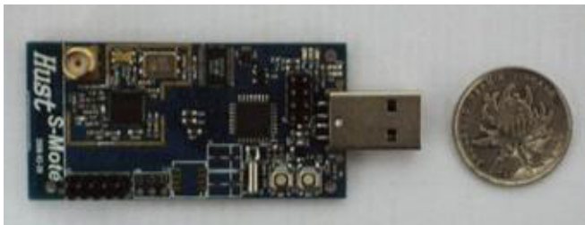
Fig. 2. The mote designed for S-Mote
