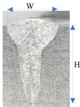
Fig. 1. The typical cross-section shape of electron beam welding of 1Cr18Ni9Ti
