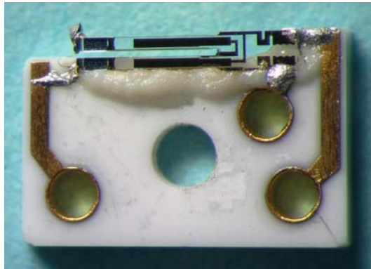
Fig. 6.10. Third generation qPlus sensor. A different ceramic substrate is used that allows to isolate the tip potential from the electrodes of the sensor. The tip is contacted with a squeezed gold wire (diameter 10\ \mu\text{m} ). The Q -value still remains on the order of a few thousand. The two electrodes of the tuning fork are fed into a single amplifier, see Sect. 6.2.4
