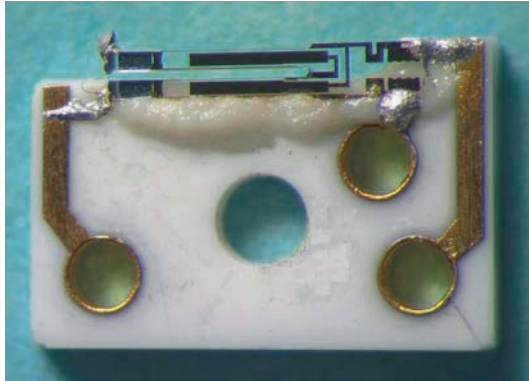
Fig. 6.10. Third generation qPlus sensor. A different ceramic substrate is used that allows to isolate the tip potential from the electrodes of the sensor. The tip is contacted with a squeezed gold wire (diameter 10\ \mu\text{m} ). The Q -value still remains on the order of a few thousand. The two electrodes of the tuning fork are fed into a single amplifier, see Sect. 6.2.4
