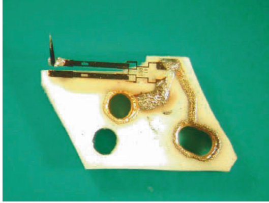
Fig. 6.9. Second generation qPlus sensor. The sensor consists of three parts: the tuning fork, a ceramic substrate, and the tip. Electrical connections are made using conductive epoxy [38]
