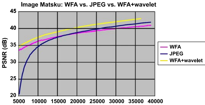
Fig. 7. The rate-distortion comparison of JPEG, WFA compression, and WFA compression of the wavelet coefficients
