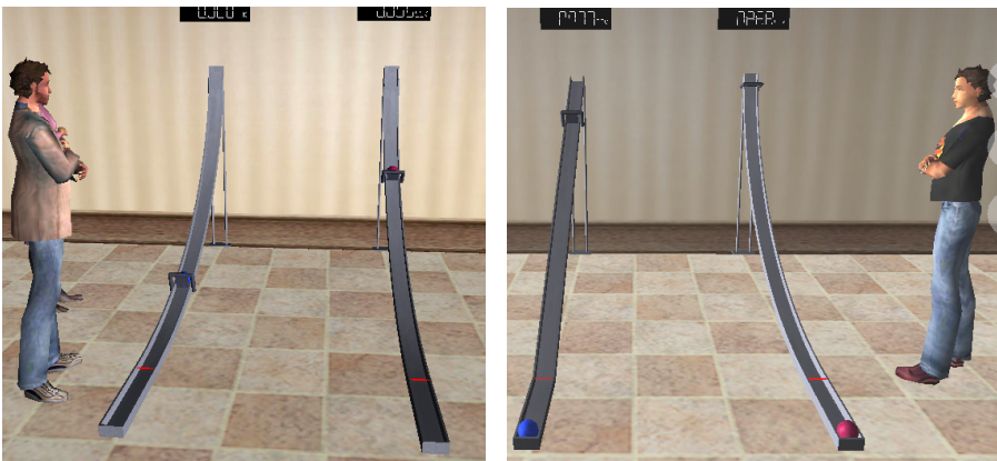
Fig. 5 and Fig. 6. Brachistochrone – inverted cycloid versus a straight line with the same endpoints; tautochrone – the ball will take a constant time to roll to the end point, regardless of its starting position
