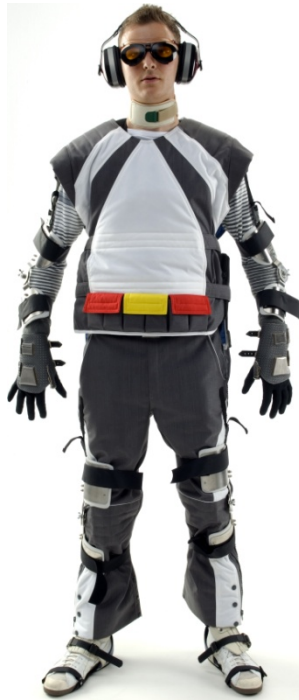
Fig. 36.12: The Chemnitz MAX, an age suit to experience effects of the elderly
