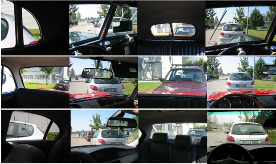
Fig. 36.6: Vision conditions during a parking activity; on top a car of the 1930s (BMW 335), in the middle a car of the 1960s (BMW 2000), on the bottom a present car (BMW 540i)
