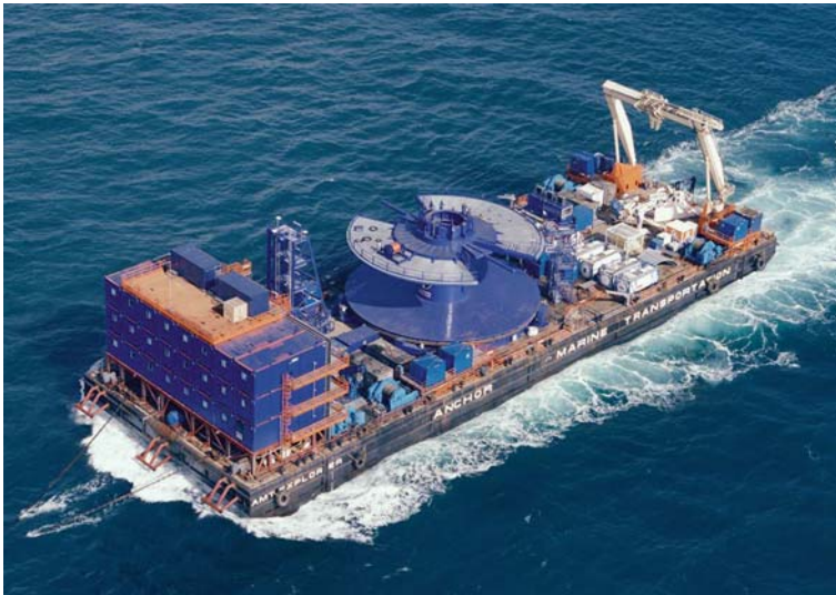
Fig. 7.2 Large cable laying barge (Courtesy of Oceanteam Power and Umbilicals, UK)
