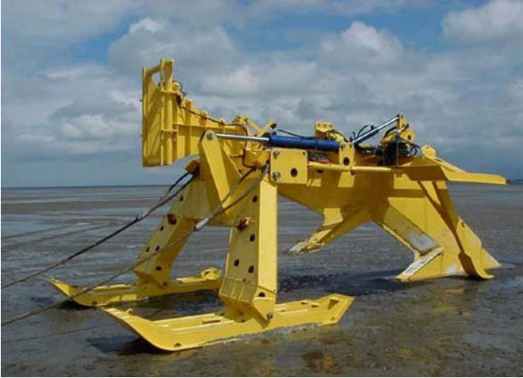
Fig. 7.24 Cable plough. The tiltable plough share to the right is now horizontal, ready for tilting down to the vertical position (Courtesy of IHC Engineering Business Ltd., UK)
