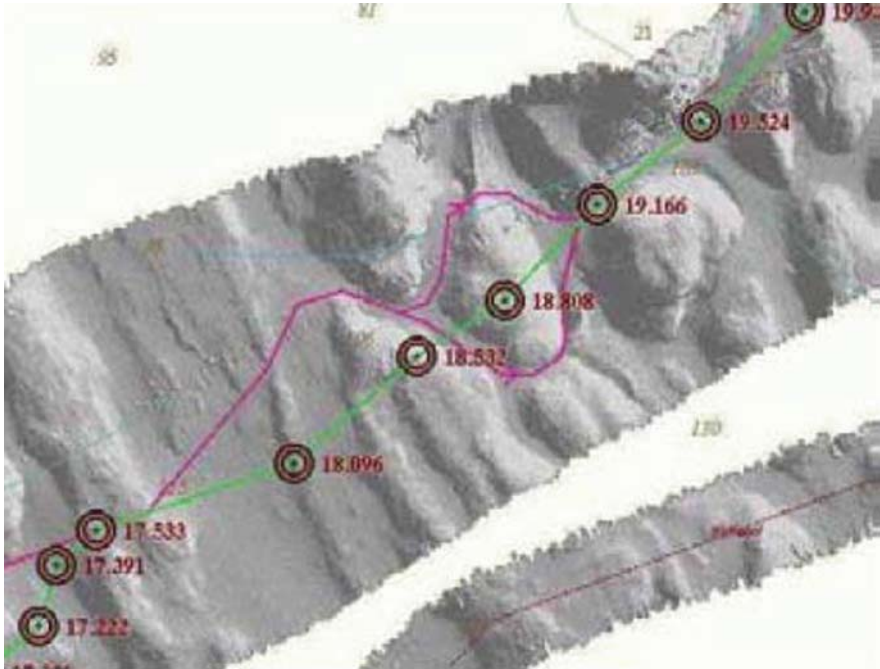
Fig. 7.22 The initially planned route ( straight line ) would have implied several ridge/valley crossings with risk for free spans. Detailed route survey enabled to lay the cable along the curved route avoiding strong undulations [12] (Courtesy of Submarine Telecom Forum)
