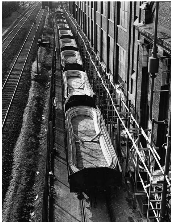
Fig. 7.12 Transport of submarine cable on railway cars (Courtesy of NKT Cables A/S, Denmark)
