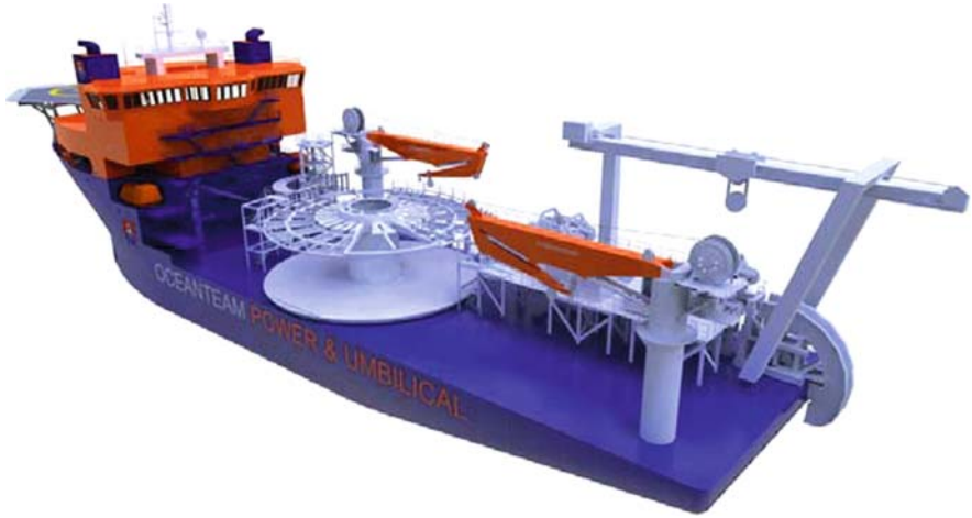
Fig. 7.5 Latest generation cable laying vessel (under construction). (Courtesy of Oceanteam Power and Umbilicals, UK)
