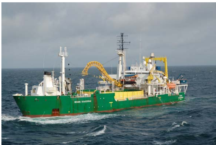
Fig. 7.1 C/S “Skagerrak” DP2 vessel with over 6000 t turntable, suitable for all kinds of power cable installation and repair
