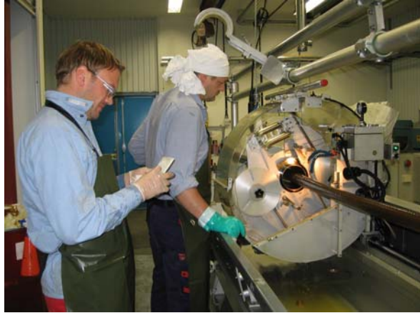
Fig. 4.2 Application of paper insulation for a flexible joint using a semi-automatic lapping machine (Courtesy of ABB, Sweden)
