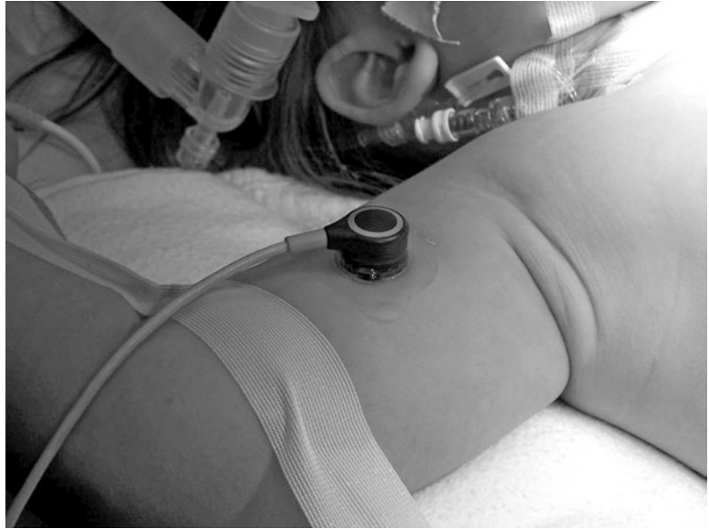
Fig. 12.13 Transcutaneous CO 2 electrode with membrane in use on a patient
