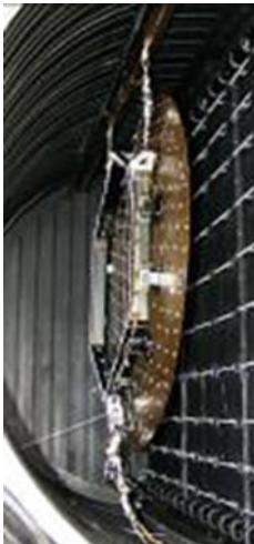
a b ■ Fig. 45.29 Astrium antenna reflector in a vacuum chamber
