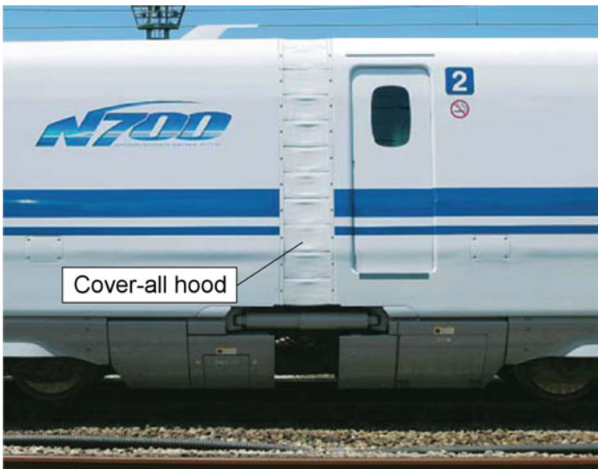
Fig. 47.8 Cover-all hood used in N700 series Shinkansen car (Central Japan Railway Company 2009b)
