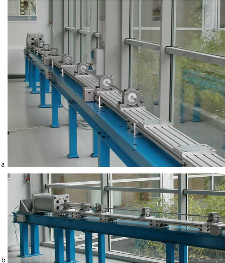
■ Fig. 21.6 Split Hopkinson Pressure Bar: (a) overall view; (b) detail of firing system and first bar (Politecnico di Torino – Vercelli Lab)
