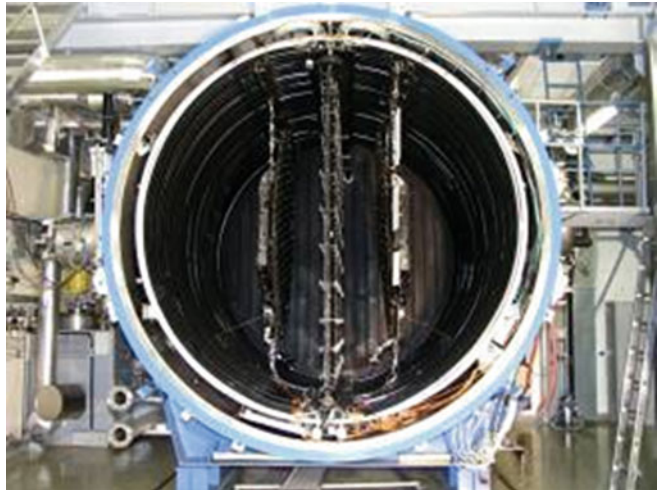
a b ■ Fig. 45.29 Astrium antenna reflector in a vacuum chamber
