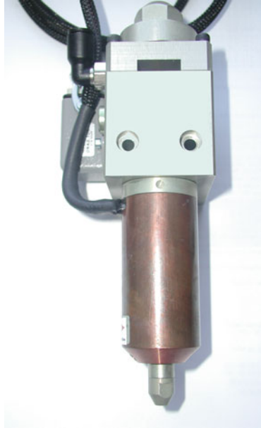
■ Fig. 37.26 Gun system to apply one-part adhesives
