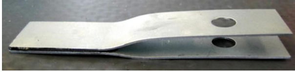
■ Fig. 46.12 Impact peel test specimen
