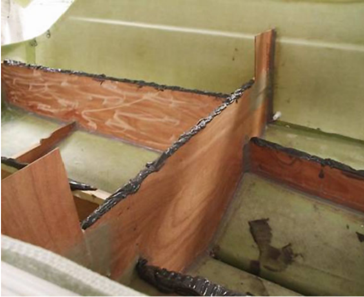
■ Fig. 48.3 Adhesively bonded marine plywood bulkhead in 6 m motor boat
