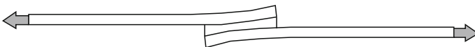
Fig. 25.8 Rotation of overlap after application of load in a single lap joint
