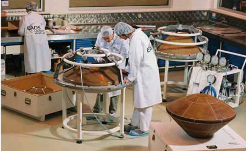
■ Fig. 45.14 Beagle 2 heat shield assembly
