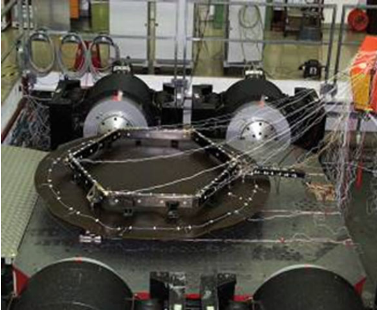
■ Fig. 45.28 Astrium antenna reflector on a sine platform test
