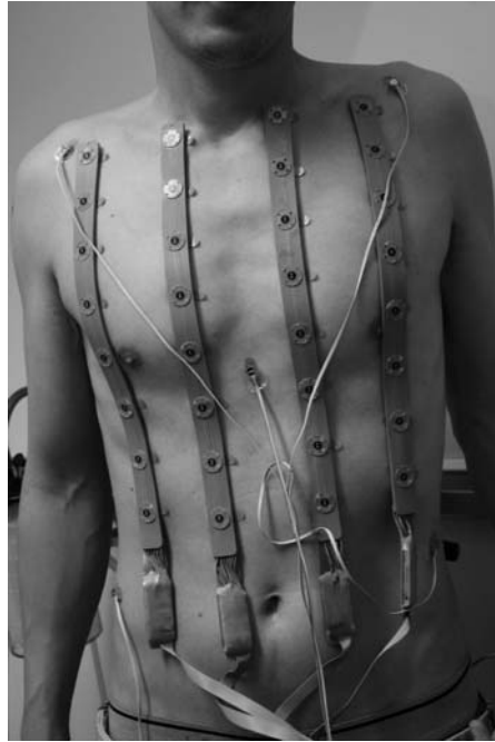
Figure 21.1 ECG equipment with 64 electrodes. Photo: Simula Research Laboratory.
