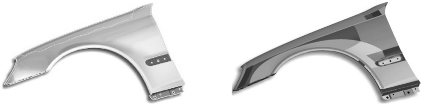
Fig. 1. Automobile sheet metal forming part with several items. Left: Manufactured and processed part at the end of a press line. Right: A geometry analyzer detects several items of a designed part.
