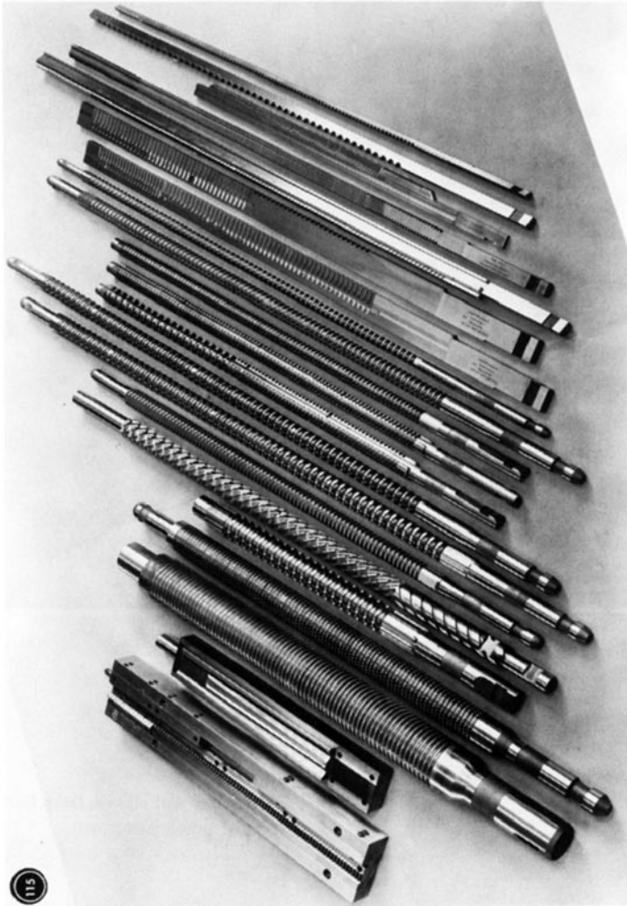
Figure 12.12 Broach types for internal- and external broaching (photo by Karl Klink, Niefern)
