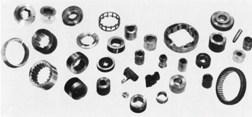
Figure 12.2 Broaching profiles for internal broaching (photo by Karl Klink, Niefern)
