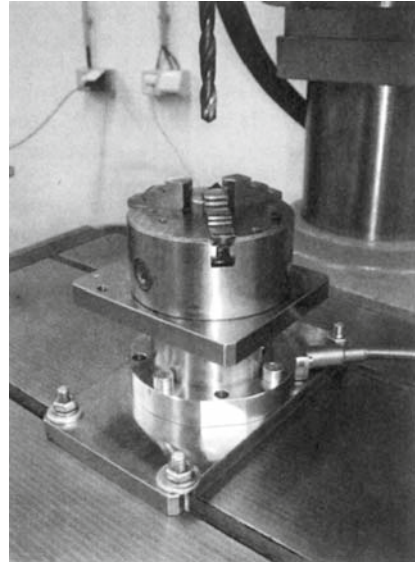
Figure 22.6 Experimental setup of force- and torque measurement during drilling (photo by HTW Dresden, practical cutting course)
