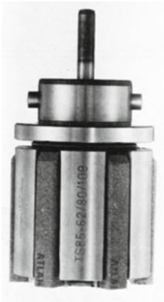
Figure 16.1 Honing tool equipped with 6 honing stones (photo by Gehring, Ostfildern)
