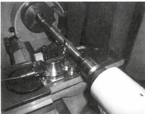
Figure 22.3 Test installation for cutting force measurement during turning (photo by HTW Dresden/Kistler AG)
