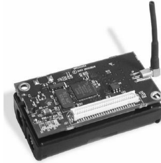
Fig. 7. MICAz mote used for localisation sensor
