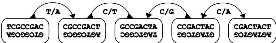
Fig. 2. The four ways in which k -molecule nodes can be connected in the bidirected de Bruijn graph of the data, with the corresponding edge labels that will be used in creating the string graph
