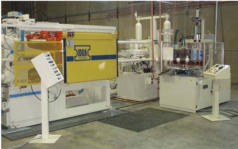
Fig. 9.1 Example of a modern 400 ton horizontal semisolid metal casting machine, and carousel induction heater
