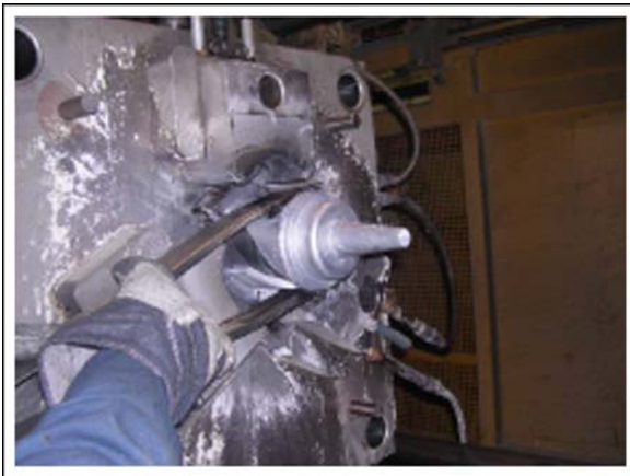
Fig. 13.15 Some die cast dies can be converted to SSM forming provided the gating is acceptable for SSM die design as discussed above. This centre-gated die was converted relatively easily and runner volume saved by moving the shot position to dead centre (Vforge)
