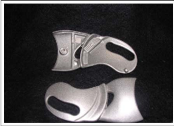
Fig. 13.14 Orthopedic knee joint piece replaced an investment cast steel piece saving 0.25 lb weight per knee! Alloy 357-T5 (Vforge)
