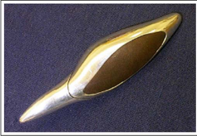
Fig. 13.10 Decorative pen and cover SSM formed from aluminium alloy 6061 in order to achieve a very high lustre polish. Aluminium alloy 357 polished to a low lustre finish because of the silicon content, and so this was one of the very first wrought aluminium alloy production applications (courtesy Vforge)
