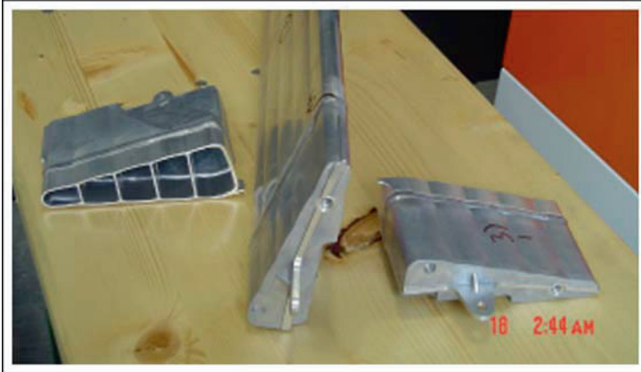
Fig. 13.8 Air tank side parts for extruded tank profile; operating pressure 16 bar, very thin walls, 240 g each part using the MHD route. Material: New alloy, high YS (290 MPa) and E 12 (%) no H.T, low porosity, weldable, Audi. (Courtesy of SAG GmbH)
