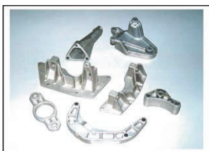
Steering knuckle, 2.2 kg, A357, T5. Substitution of cast iron part for Alfa Romeo
