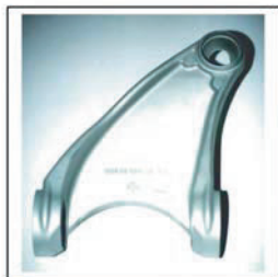
Steering knuckle, 2.2 kg, A357, T5. Substitution of cast iron part for Alfa Romeo
