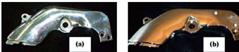
Fig. 11.6 (a) Polished swing arm mount from Figure 4.21 (a), and (b) Chromium plated SSM cast part.
