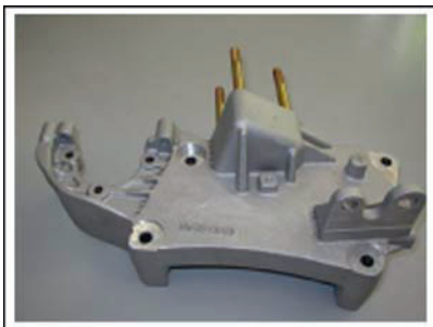
Fig. 13.7 Rheocast high strength safety parts: engine bracket ( left ) and Lagerbock ( right ) both using A 357 alloys (courtesy of Stampal S.p.A)
