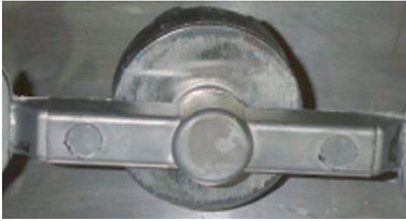
Fig. 11.1 Representative diaphragm style to minimise slug surface oxide entering the die cavity [10]
