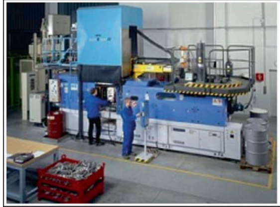
Fig. 13.2 220t-Thixomoulding ® -machine from Japan Steel Works at Neue Materialien Fürth GmbH (NMF)
