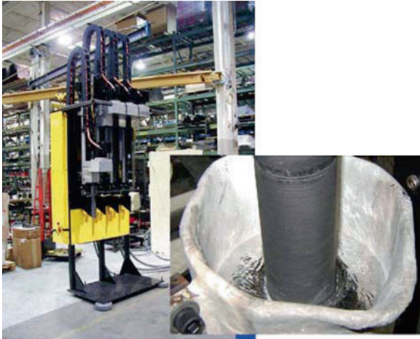
Fig. 10.11 SSR cell and graphite stirring rod in melt
