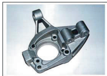
Front Suspension arm (L&R), 600 gr, A356, T6. Substitution of forged part for TRW
