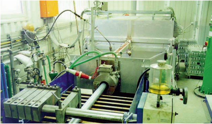
Fig. 10.1 Mini horizontal continuous caster equipped with electromagnetic stirrer shown casting 75 mm SSM diameter billet, courtesy Hertwich GmbH
