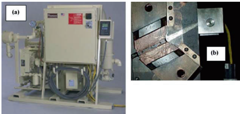
Fig. 11.4 (a) Die vacuum system with 7.5 HP pump and 113.55L tank and (b) Vacuum runner for the part shown in Figure 11.5
