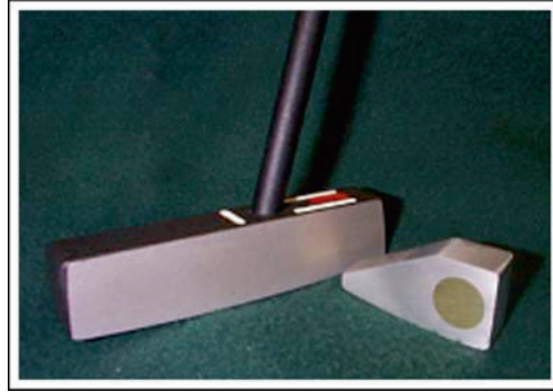
Fig. 13.12 One of the very first SSM copper alloy production parts. A golf driver sole plate formed from aluminium bronze alloy replacing a stamped and machined alloy 377 piece. This application offered improved wear resistance from the superior alloy as well as a near net-shape without machining requirements (Vforge)
