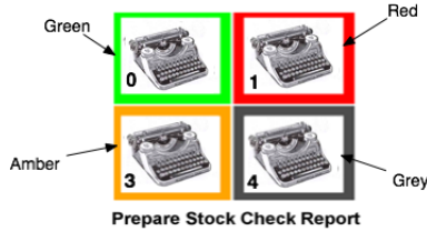
Fig. 10. Illustration of an aggregated icon made up of single task icons. The example shows a task titled "Prepare Stock Check Report" with zero checked in, one checked out, three available and one task unavailable. The colour of each segment is annotated beside the icon for clarity.
