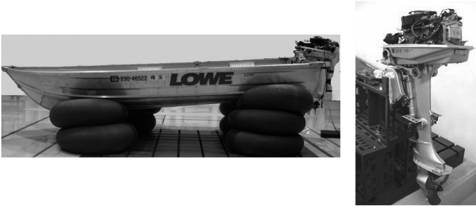
Fig. 1 The Boat-Hull and the Outboard-Engine with Its Suspension-Mechanism to Be Tested
