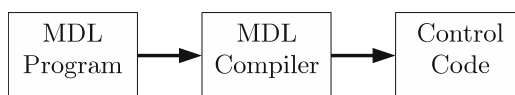
Fig. 1. An illustration of the process of turning high-level MDL programs into executable control code
