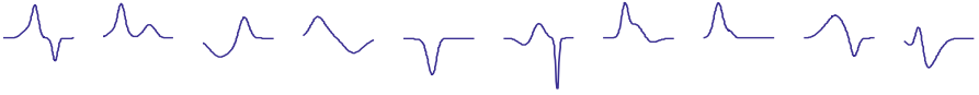
Fig. 3. 10 examples of randomly generated evoked responses using a mixture of 3 Gaussian shaped time signals
