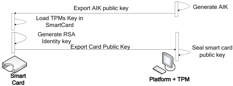
Fig 2. Cryptographic Binding of the TPM and Smart Card
