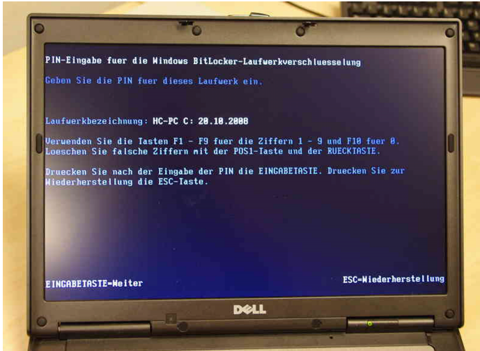
Fig. 1. Spoofed BitLocker PIN-entry screen
