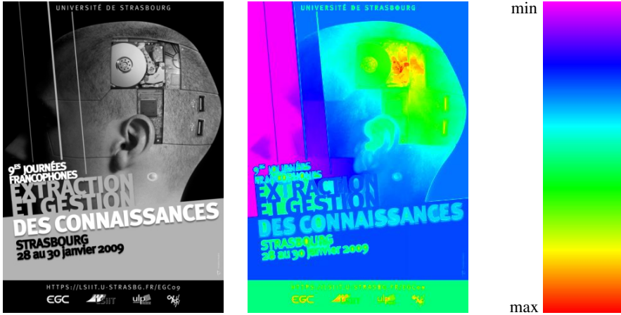
Fig. 2 Illustration of the topographical distance computed from the top-left pixel (from left to right): input image, topographical distance transform, look-up table representing the distance scale
