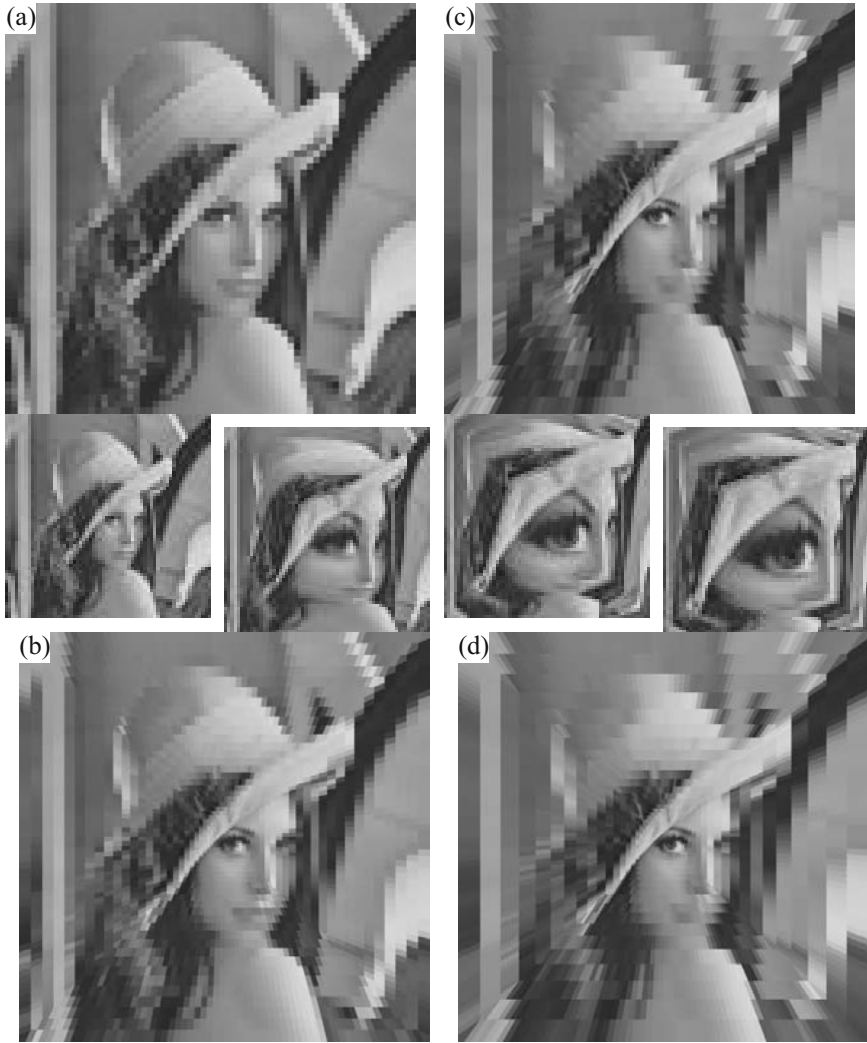
Fig. 4. Comparison of the different mappings using the L_\infty mapping method: the small images are the foveated images, and the large images have remapped them back onto the original. (a) uniform downsampling to (64 \times 64) ; (b) mapping of Eq. (11); (c) mapping of Eq. (12); (d) mapping of Eq. (13).
