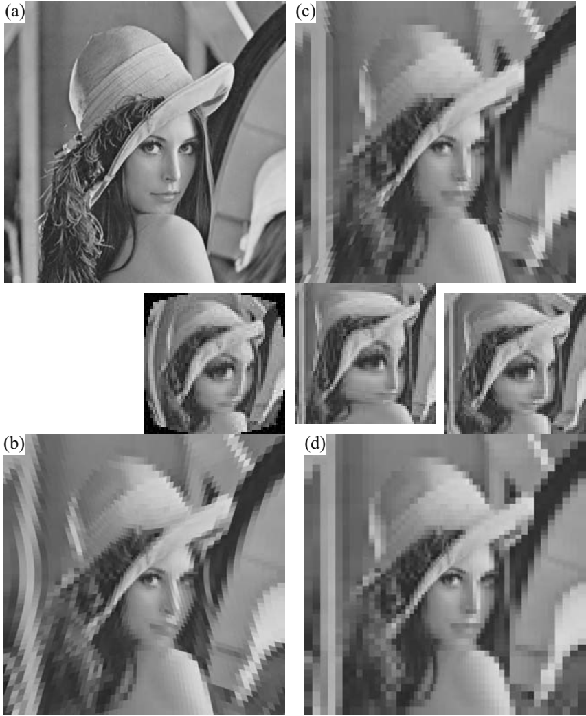
Fig. 3. Comparison of the different mapping methods: the small images are the foveated images, and the large images have remapped them back onto the original to show the acuity. (a) original Lena (512×512); (b) radial L_2 mapping; (c) radial L_\infty mapping; (d) separable mapping.
