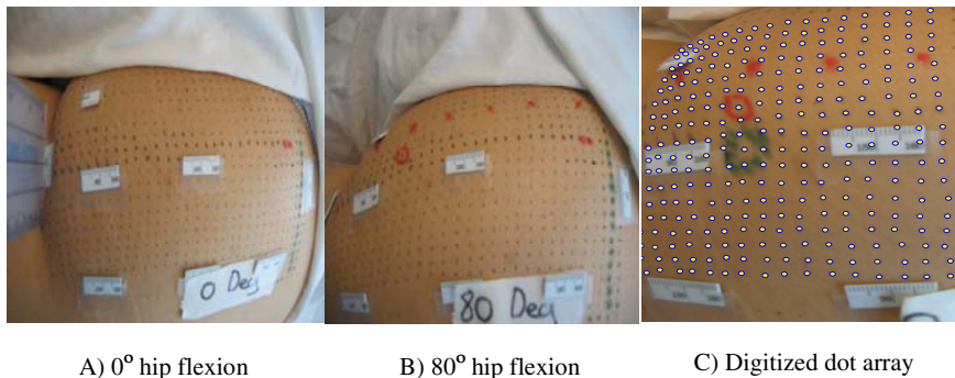
Fig. 9. Measurement of buttock skin initial tensile strain induced by a sitting posture relative to a standing posture
