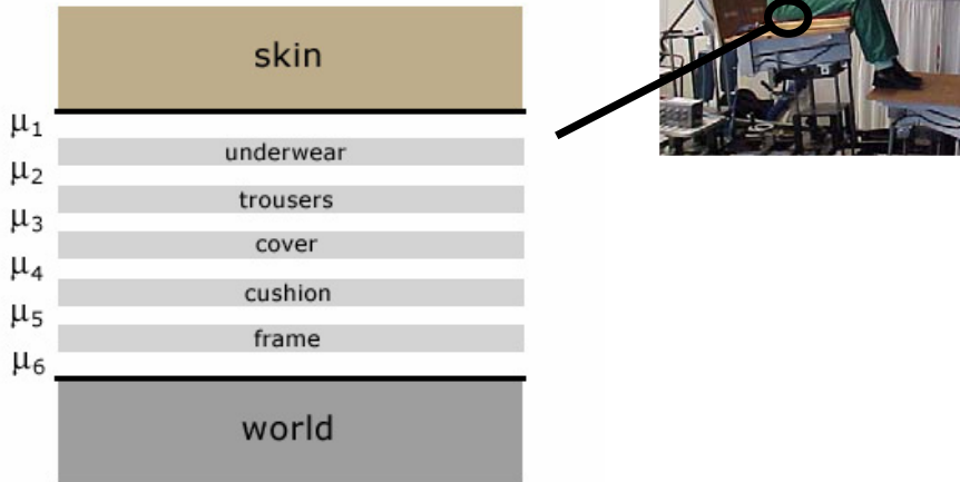
Fig. 7. Different layers at the interface. From skin to world contains 6 surfaces that make contact. Each two surfaces with their own coefficient of friction.
