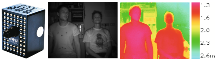
Fig. 1. Near-infrared intensity image (middle) and color coded range image (right) captured by the 3-D camera SwissRanger SR-3000 (left, [22])
