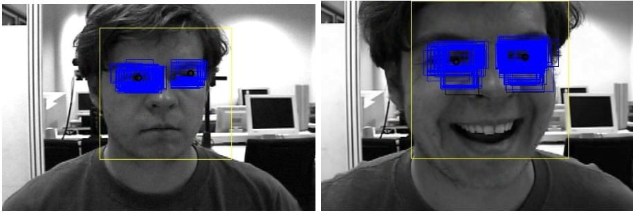
Fig. 6. Our localization algorithm yields a region of interest for the face and also determines the positions of the eyes within a second application of the Viola and Jones approach as indicated by these two exemplary images. This information is now used to roughly parameterize the face model.
