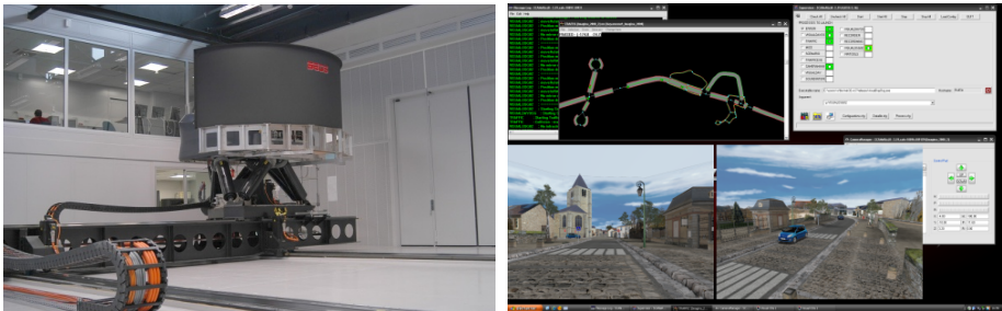
Fig. 5. The dynamic simulator Ultimate at Renault ( left ), and a screenshot of the SCANer™ software with two visuals outputs, the traffic and the supervisory modules ( right )
