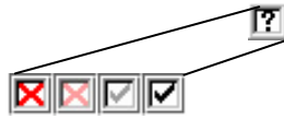
Fig. 5. Clicking on the checkbox turns it into four choices whose tool tips say “it’s wrong,” “seems wrong maybe,” “seems right maybe,” “it’s right.” [3]
