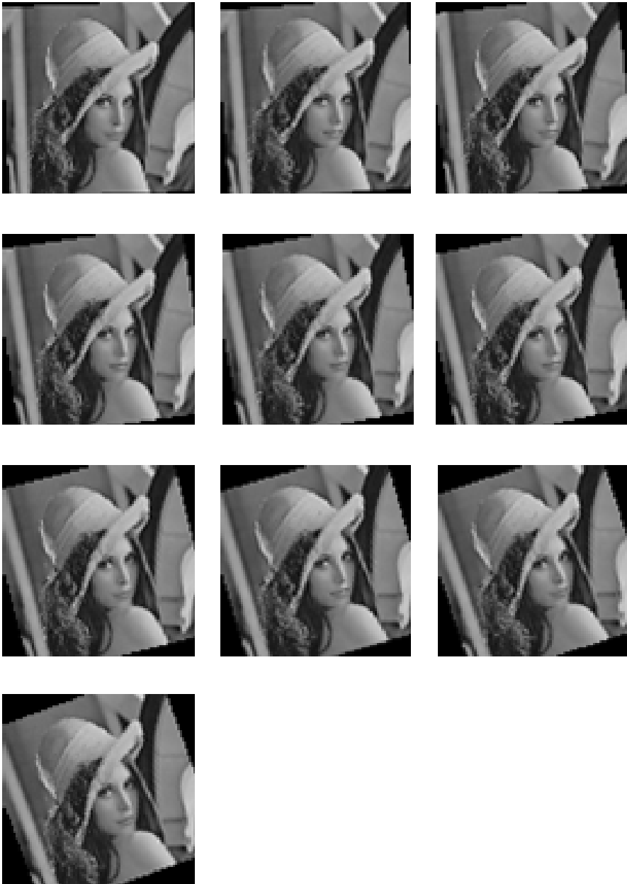
Fig. 5.2 Rotationally and translationally shifted noiseless low-resolution frames [85 x 85], of the 'Lena' sequence
