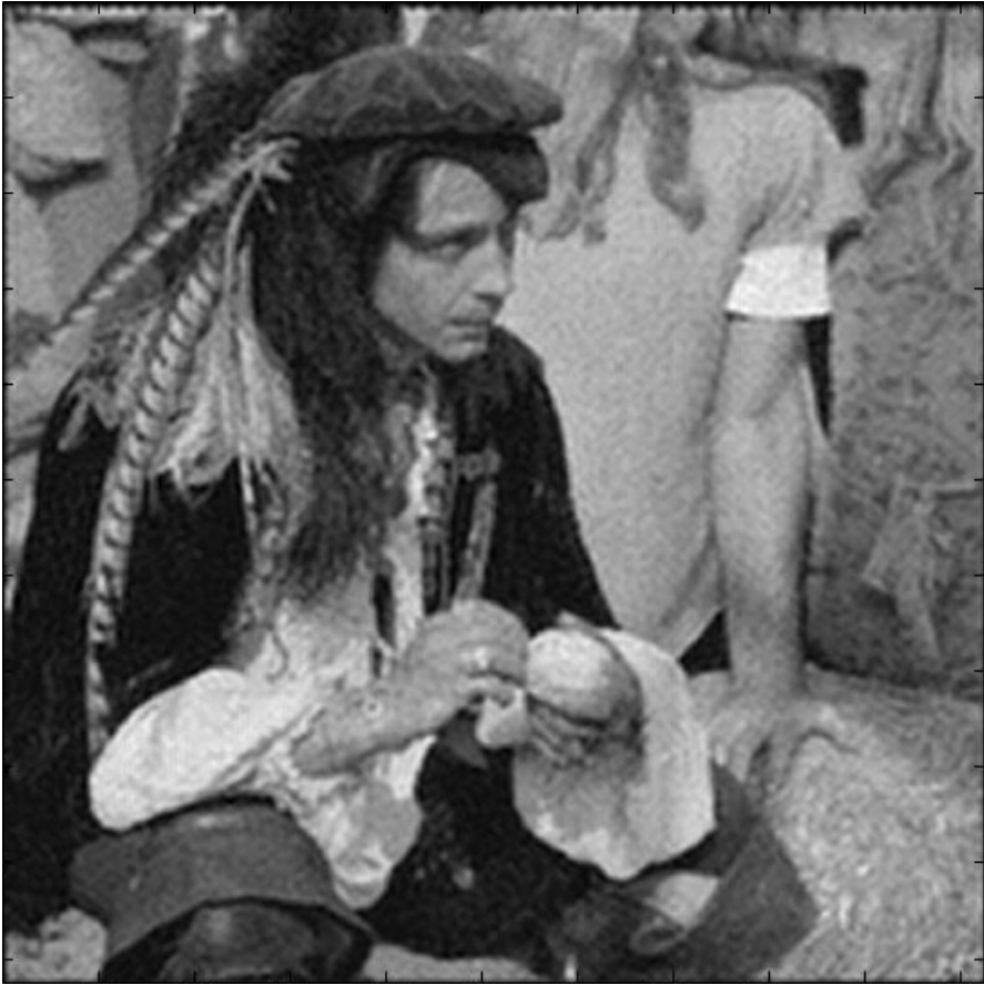
Fig. 3.14 IISR-generated high-resolution image from only 10 noise corrupted LR frames of the ‘man’ sequence [1024 x 1024] with an E_{rmse} = 0.17301 and E_{psnr} = 63.3696 dB
