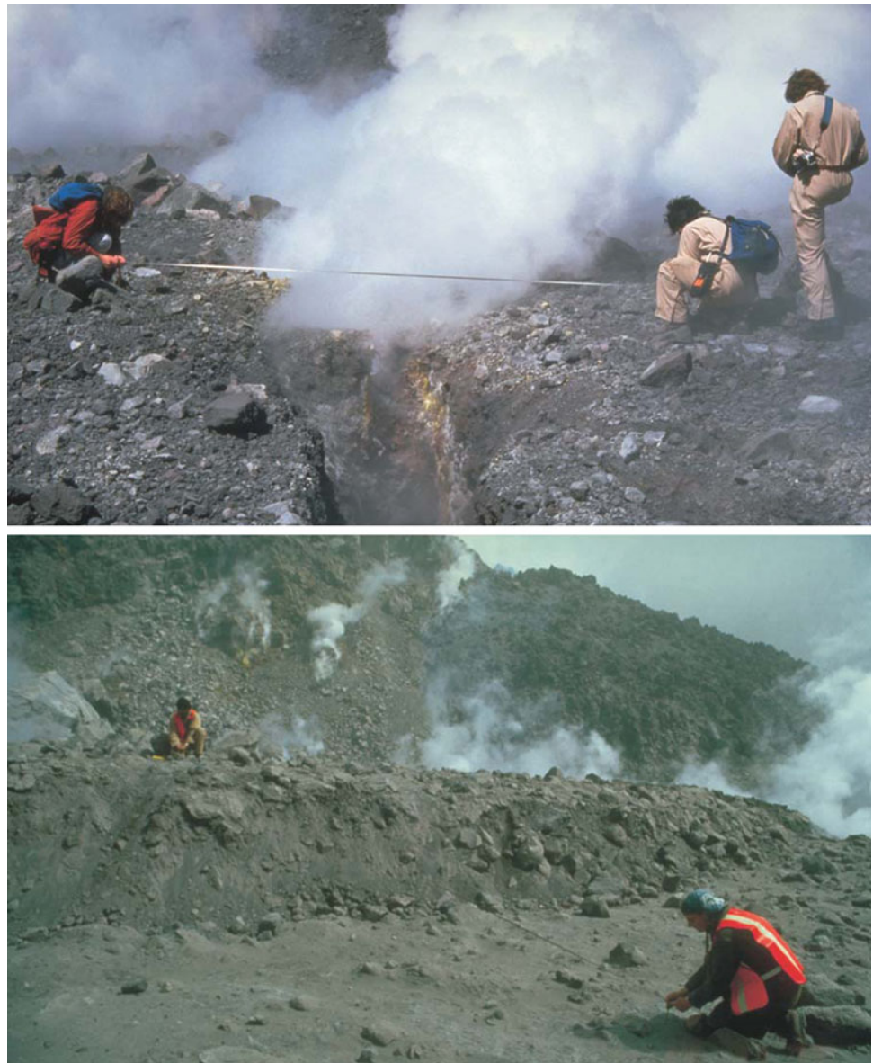
Fig. 5.1 Scientists measure displacement across a radial crack ( top ) and circumferential thrust fault ( bottom ) on the crater floor at Mount St. Helens. USGS photographs taken by Lyn Topinka on 12 May 1984 and by Terry A. Leighley in 1981, respectively
