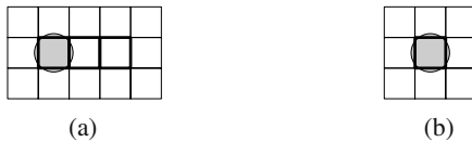
Fig. 7. The sizes of a mixer and a storage unit. (a) A mixer with 3 electrodes for droplets to move. S_{mix} = 15 . (b) A storage unit with 1 electrode for droplets to stay. S_{store} = 9 .
