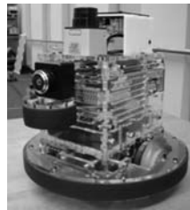
Fig. 3. Scarab, differential drive robotic platform, outfitted with a camera, Urg laser unit and tracking beacon.
