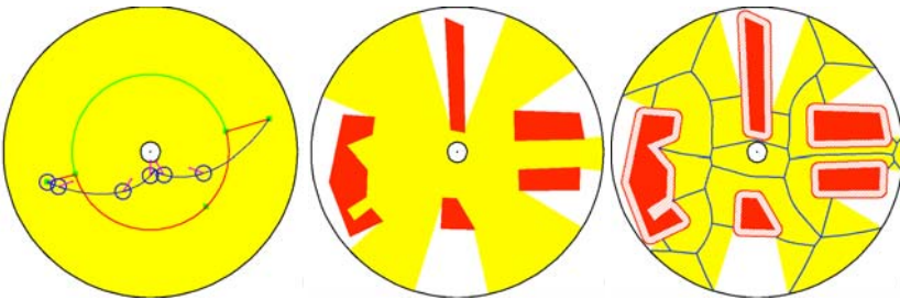
Fig. 6. (Left) Shortest paths for a DDR under visibility constraints alone (angular and distance ranges, represented by the inner and outer circles). The robot shape, heading, and gaze are drawn here, and then omitted for the sake of readability. The Voronoi-based path is in dark, so is the final computed path. (Center) Obstacles (dark) and regions visible from the landmark (light gray). (Right) Construction of \mathcal{C}_{free}^g : dilated obstacles (dashed grey) are removed from the visible area and underlying GVG.
