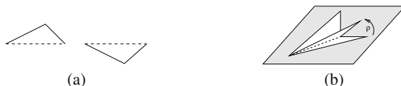
Fig. 5. (a) In 2D, the same vlink represents two configurations: a concave and convex triangle. (b) In 3D, the same vlink represents many configurations with different dihedral angles \rho .
