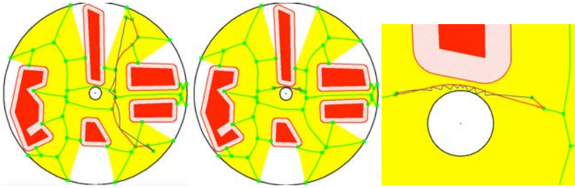
Fig. 7. (Left) Examples of a path computed by the recursive algorithm. (Center) and (Right) Behavior of the planner in narrow passages: as expected, a solution may imply a quantity of maneuvers to finally reach the goal. (Right) is a zoomed view of (Center).
