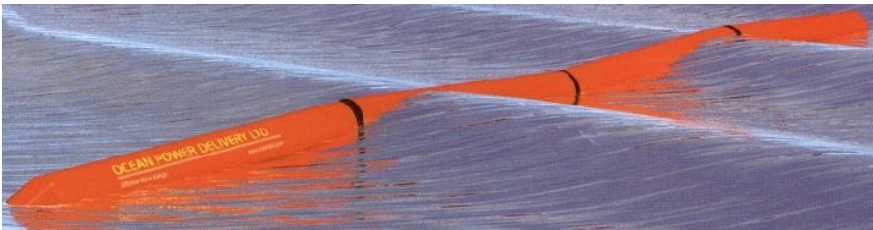
Fig. 7 The Pelamis, a wave energy converter developed by Pelamis Wave Power Ltd. It resembles the lamprey (in fig. 4a), both visually and in locomotion.
