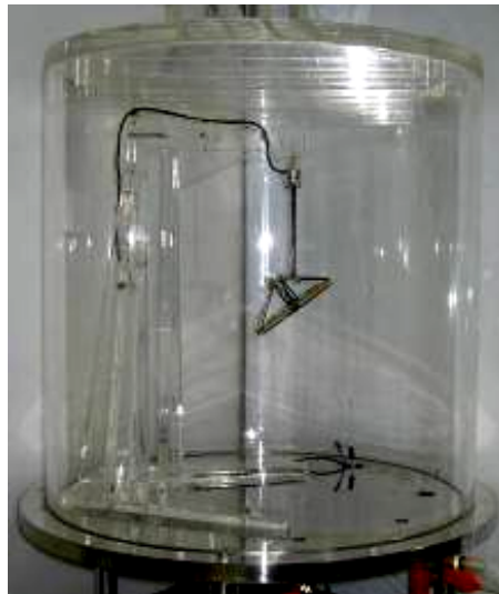
Fig. 10. Force measurement in the vacuum
