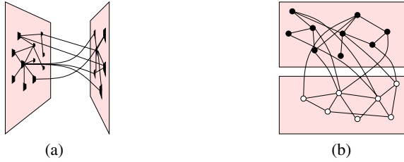
Fig. 1. Schematic illustrations of a visualization (a) adopted by VisLink, (b) using different semantic substrates of a same network. In both the visualizations the drawing on each plane has been computed without taking into account the relationships with the other. This may cause many crossings between inter-sets relationships.
