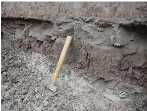
Fig. 12.17 An incompetent bed at the north side of Shalong Road, Sanwan pool, Wanzhou
