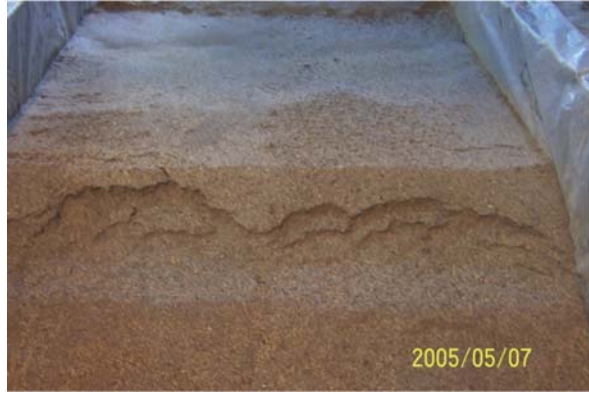
Fig. 27.7 Bank collapse for the erosion type
