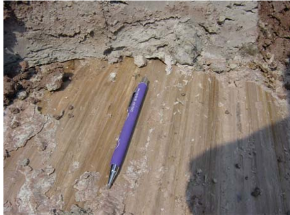
Fig. 12.7 The striations of Y2 slip zone of the Anlesi landslide (the sliding direction is 102°)
