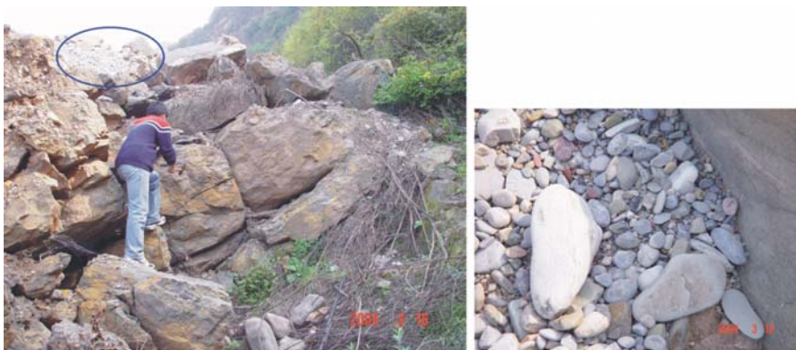
Fig. 8.7 Gravels displaced from the bed of Qinggan-he River and deposited in the toe of the landslide deposit (circled in photograph). Note that the sandstone dip direction is reversed and the dip angle has become steeper compared with Figs. 8.4 and 8.5)
