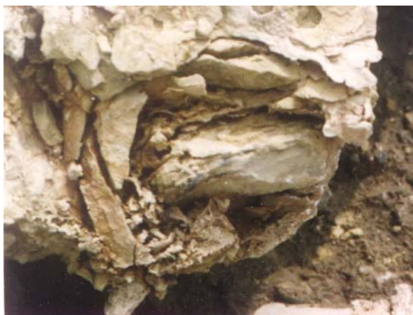
Fig. 3.17 Breccias at the shearing outlet in the front edge of the Huangtupo landslide, a shredded cabbage pattern occurs as a result of strong pressure, in the riverfront, 300 m to the east of Sidaogou
