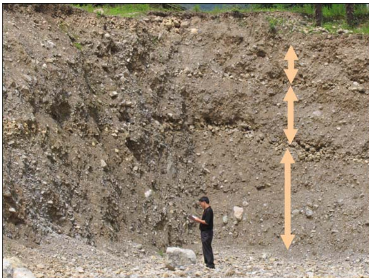
Fig. 13.5 Part of the section showing the structure of the Yangjiawan mud-rock flow deposits. Each layer was made up of a thinner coarse layer and a normal one (the man is about 1.7 m tall)
