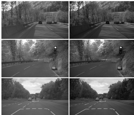
Fig. 1. Examples of stereo pairs of Set 1 on the enpeda.. test sequence website (from Sequences 5, 6, and 7, recorded with 12-bit Bosch night vision cameras)
