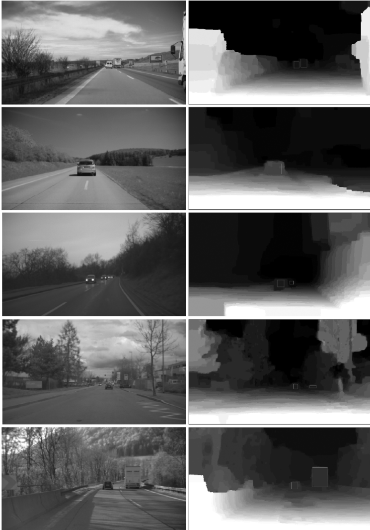
Fig. 10. Examples of manually specified rectangular regions for approximated ground truth: in original sequences (left) and in Sobel-based BP results (right)
