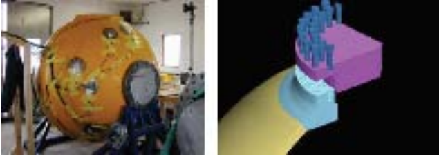
Fig. 3. Hydrodynamic containment vessel (LANL Weapons Engineering)
