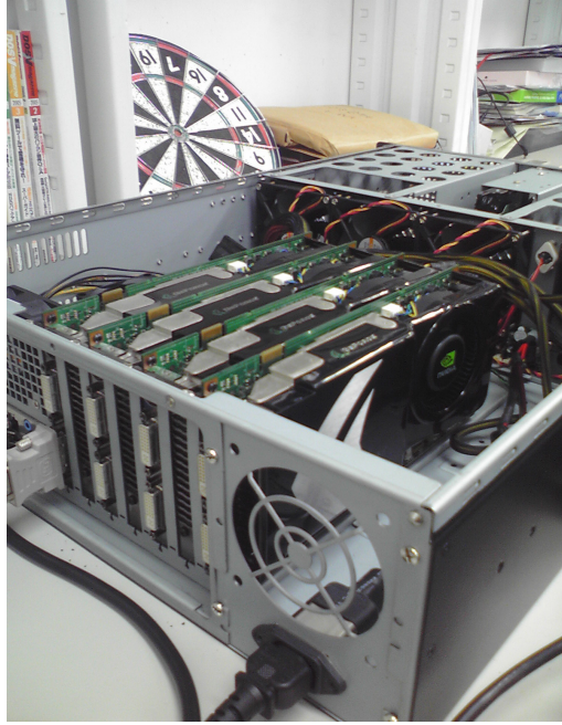
Fig. 4. A 3U Compute Node with 4 Nvidia 8800GTS cards
