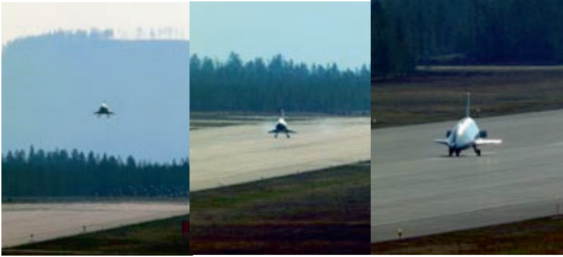
Fig. 3.28. PHOENIX demonstrator: Test of subsonic free flight (helicopter drop test) and landing capability in Vidsele, Sweden in May 2004.
