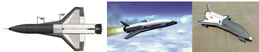
Fig. 3.21. X-34 shape: planform view (left) [26], synthetic image (middle), X-34 on NASA Dryden ramp (right) [27].
