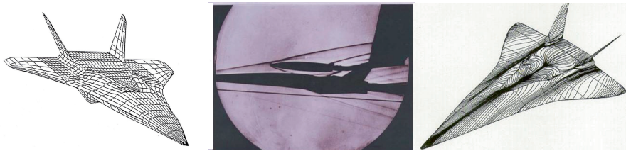
Fig. 4.19. SÄNGER configuration without HORUS Orbiter: panel grid (left) [18], and skin-friction lines evaluated from a Navier–Stokes solution (right). The figure in the middle shows a wind-tunnel schlieren picture of the stage separation process [22].
