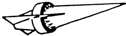
Fig. 4.38. Schematic of a (zero angle of attack flight) scramjet accelerator vehicle with conical forebody and circular inlet/engine arrangement [1].
