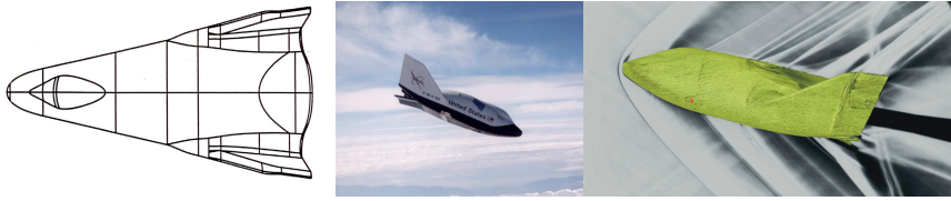
Fig. 3.23. X-38 shape, Rev. 8.3, planform view (left), vehicle #2 in free flight (middle), [27], model in wind tunnel (right) [30].
