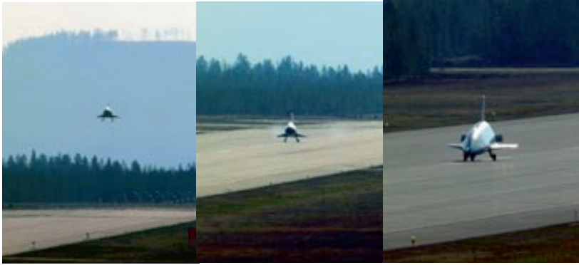
Fig. 3.28. PHOENIX demonstrator: Test of subsonic free flight (helicopter drop test) and landing capability in Vidsel, Sweden in May 2004.
