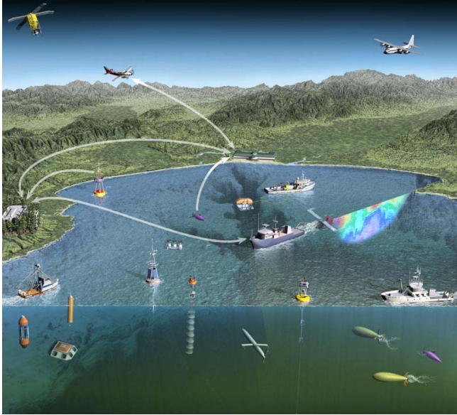
Fig. 1. Artist’s rendering of intensive observational campaign to observe the waters of Monterey Bay with a variety of platforms. Data from these platforms are transferred to shore for processing and in some cases products are transferred back to shipboard teams.
