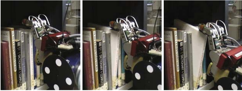
Fig. 6 The robot grasping the book by means of force and tactile-based continuous estimation of hand-to-object relative pose
