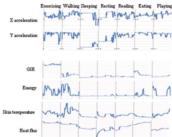
Fig. 5 The Raw Sensor Data from the Accelerometer and Significant Physiological Signals of Each Activity
